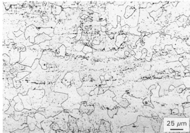
Figure 1 Optical micrograph showing the microstructure of AISI 430 steel in the as-received (skin-pass) condition (parallel to the rolling plane).
